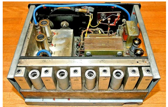
Top view of a Sázava II (TI-457-1) showing RF front end unit (top left with two valves on a silver plated enclosure); AC mains power supply and AF output stage (top right); IF strip (bottom).
