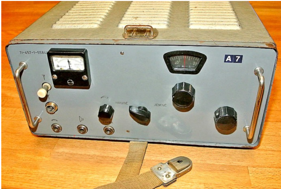
Front panel view of the Sázava II (TI-457-1). A meter with a centre scale pointer allowed accurate tuning to the FM signal of a bug.
